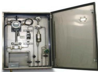
Housed in a stainless steel enclosure, the basic Sarasota SG901 system comprises a Thermo Scientific Sarasota FD900 gas density assembly, temperature element, and flow control valve. All components are binterconnected by 6.35 mm (0.25") stainless steel tubing. The basic system is ideal for applications where the analyzer is used in conjunction with an existing gas conditioning system that provides a clean, dry sample at a pressure below 4 bar A (58 psia).
